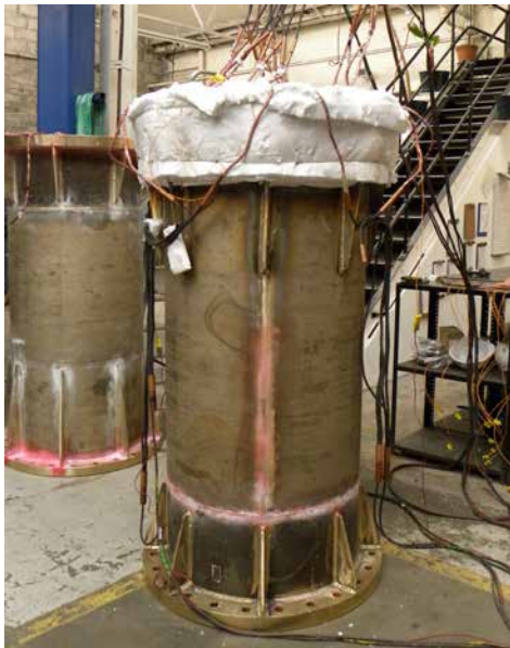
Figures 57 and 58 - Selective annealing heat treatment of a welded flange on a desalination pump housing using resistance heating elements, 675°C for six hours (Courtesy Site Heat Treatment, Port Talbot, and Copper Alloys Ltd, Stoke-on-Trent, UK)
