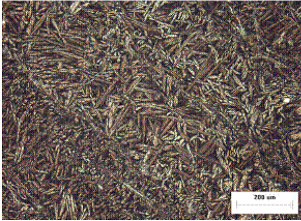
Figure 36 - CuAl10Ni5Fe4Mn DIN 2.0966 Widmanstätten martensitic structure. Water quenched from 900°C. Etched in acidified ferric chloride solution.
