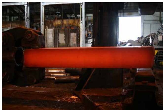
Figure 76 – Open die press forging of 5000 kg billet (Courtesy of Copper Alloys Ltd, Stoke-on-Trent, UK)
