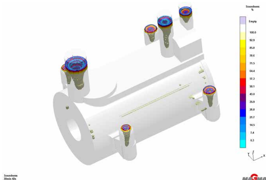
Figure 65 - Casting simulation showing a prediction for soundness (Courtesy Inoxyda SA, France)
