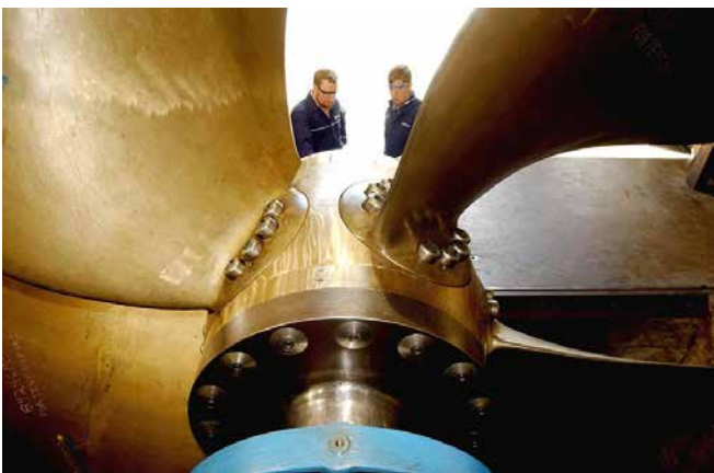
Figure 12 - Variable pitched propeller (Courtesy Rolls Royce Marine)
