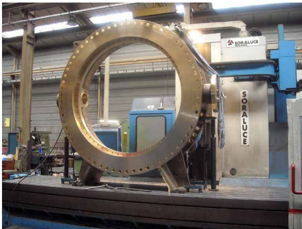
Figure 32 – Valve body 2000 mm dia 6000 kg (Courtesy Inoxyda SA, France)
