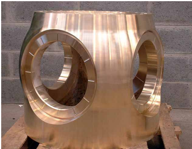
Figure 14 – Hub body 8500 kg (Courtesy Inoxyda SA, France)
