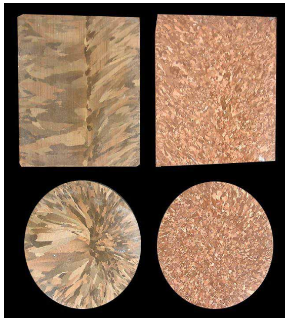
Figure 71 – Grain refining in continuous casting
